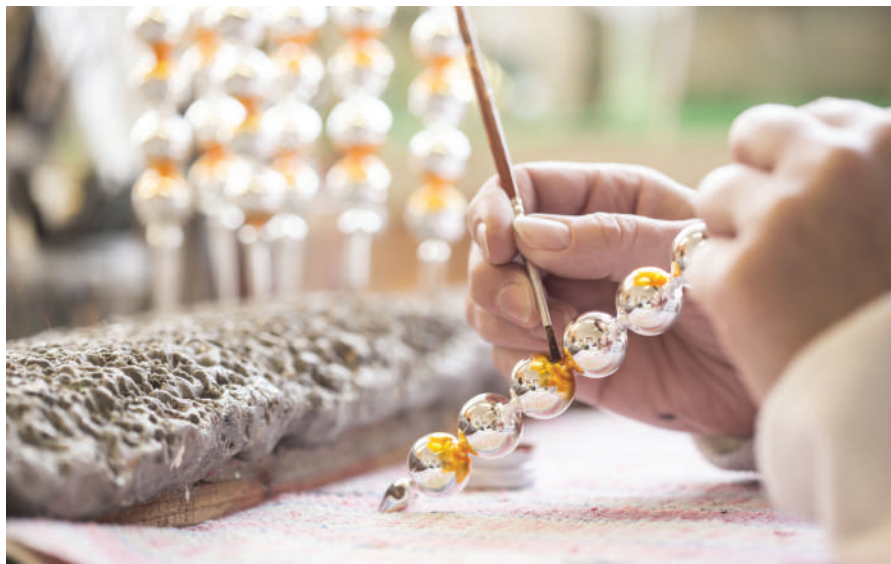
Handmade Production of Christmas Tree Decorations from Blown Glass Beads. All photos: Museum of the Bohemian Paradise in Turnov
